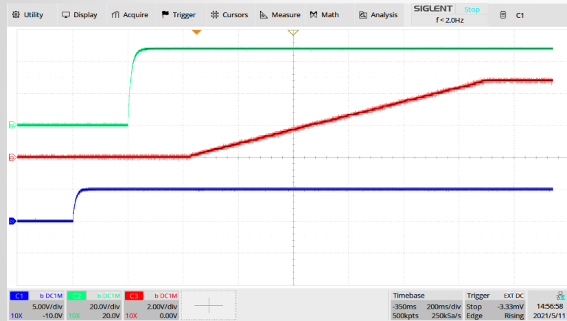
ON/OFF Delay to simulate different power-on/off sequence
