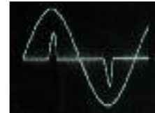
Same conditions as above with programmable Z_o engaged. THD=0.25%
