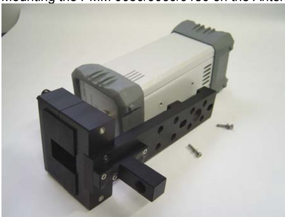
Mounting the PMM 9030/9060/9180 on the Antenna Holder
