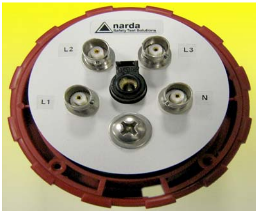
A-D-18 PMM L3-64 model adapter (64 A sockets)
