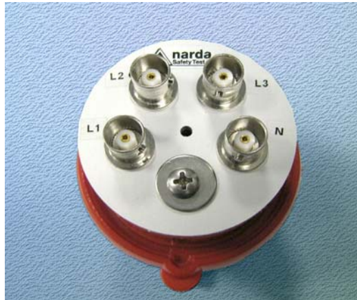
A-D-17 PMM L3-32 model adapter (32 A sockets)
