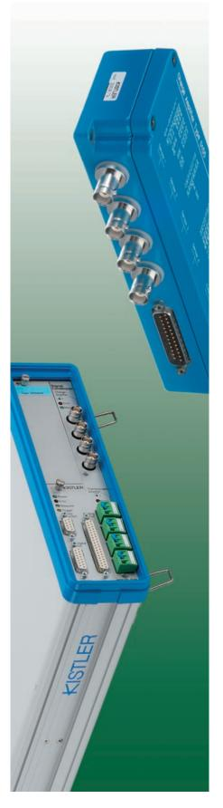
Charge amplifiers convert charges transmitted by a piezoelectric pressure sensor into a proportional voltage, which can be used as an input variable for monitoring and control processes. Kistler supplies a wide range of different charge amplifiers such as single-channel charge amplifiers or multi-channel amplifiers for charge and temperature.
