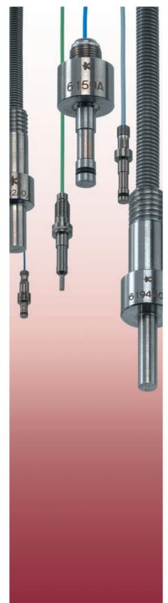
The cavity pressure built up during injection molding processes can be measured directly, indirectly or in combination with the contact temperature. During direct measurement the sensor touches the plasticized material within the cavity to determine the pressure directly, without the use of transmission pins.
