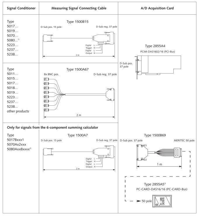
$<sup>^{1)} \</sup>text{ Cable Type 1500B15 is used when output signals } F_{x_1+z_1} F_{x_3+z_1} F_{y_1+z_1} F_{y_2+z_1} F_{z_2}, F_{z_3} F_{z_4} have \text{ to be acquired.} \\$
