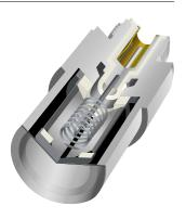
Section through a piezoelectric pressure sensor
