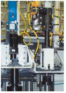
Mounting station in German automotive factory with electromechanical NC joining module NCFH
