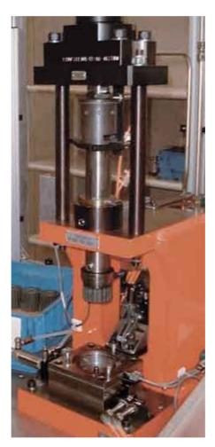
Force-displacement monitoring of press fitting of needle bearings into gearbox
