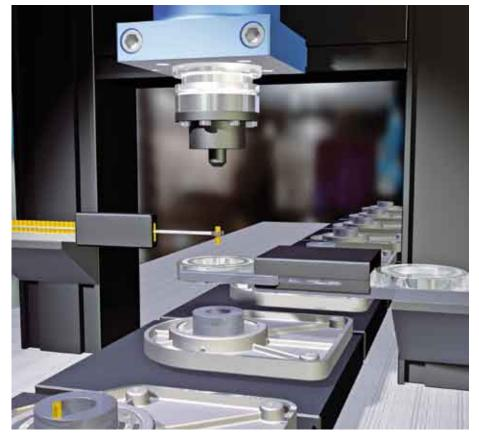
NC joining system NCFH used to press-fit bearings on Compactness of hollow-shaft motor allows 795 mm long NC joining module NCFH to offer 400 mm stroke production line
