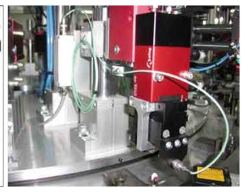
Testing spring-loaded switches for car brake or clutch pedals and accelerators with force sensors Type 9203 andcharge amplifier Type 5037B1211
