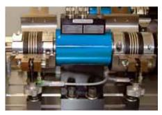
Torque sensor with base and two double-flexible couplings
