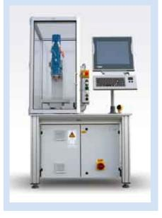
Kistler supplies piezoelectric, piezoresistive, capacitive and strain gage sensors. Piezoelectric designs are particularly suitable for measurement imposing extreme requirements in terms of geometry, temperature range and dynamics. Kistler therefore relies mainly on the piezoelectric principle for measuring dynamic forces in assembly and testing.
