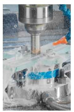
ing processes such as turning, milling, grinding or drilling. This yields significant data on the cutting, feed and passive forces involved. Preliminary analysis of cutting forces improves process capability for large-scale production. Monitoring of these forces subsequently helps detect overloading, tool collisions and tool damage.
