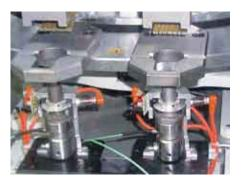
The resultant preload force is mainly dependent on the tightening torque. Kistler's piezoelectric torque sensors can extremely accurately monitor and record the torque curve of any screw connection made. By preventing overloads and prior damage to these connections, this ensures more reliable, higher-quality products.
