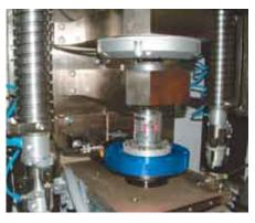
Drivetrain with torque measuring flange Type 4504A... and angle sensor
