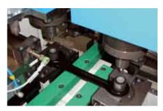
Two electromechanical NC joining systems press elastomer bushings into struts
