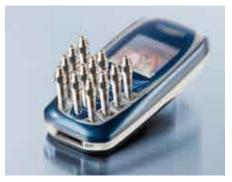
Sensor Type 9215 with an outside front diameter of only 5 mm at front for measuring minute forces. This type of sensor makes it possible to scale down miniature force plates and sensor arrays to a spacing of 7,5 mm for checking applications such as cell phone keypads at just one test station
