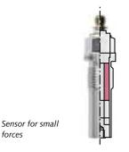
the cover plate in a welded case. The electrode located between the two guartz disks receives the measurement signal and transmits it to the connector. Load washers are sturdy and highly versatile in application. Their central hole allows easy integration into various structures in a variety of different configurations and preloading by means of a screw.
