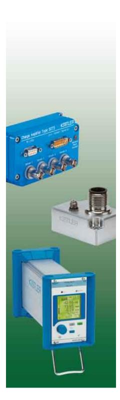
Signal conditioning is essential in measuring mechanical quantities such as force, strain or torque. **Charge amplifiers** convert the charge output by a piezoelectric sensor into a proportional voltage; whereas **strain gage amplifiers** boost the small measurement voltage signal. These voltage signals are then also used as input variables for monitoring and control processes.
