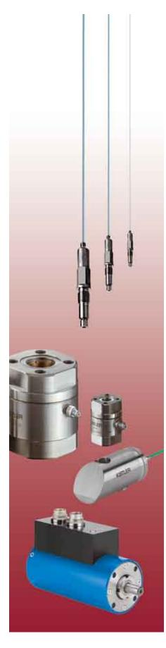
When it comes to measuring dynamic forces, Kistler mainly relies on the piezoelectric principle. Under mechanical load piezoelectric materials produce positive or negative electric charges. Charge amplifiers convert the charge generated by the piezoelectric material into a proportional voltage. Quartz disks with piezoelectric properties can be arranged in sensors to measure one or several force components or one torque vector.
