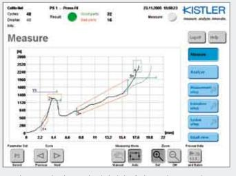
Disturbances can be eliminated with the help of relative tolerance windows
