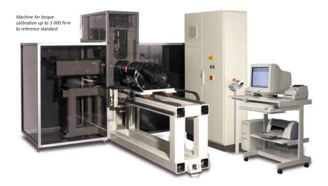
During **continuous calibration**, the load is continuously increased to the required value within a defined time and then reduced to zero within the same time. A "best straight line" passing through the origin is defined for the resultant characteristic, which is never exactly linear. The gradient of this line corresponds to the sensitivity of the sensor within the calibrated measuring range.
