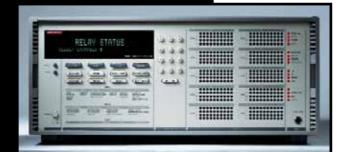
The Model 7002 Switch System is a 10-slot mainframe that supports up to 400 2-pole multiplexer channels or 400 matrix crosspoints. The front panel includes a unique interactive display of channel status for quick programming. Scanning speeds of up to 165 channels per second are possible with the high density switch cards. The wide selection of more than 30 different switch cards makes the 7002 one of the most flexible switching mainframes available.
