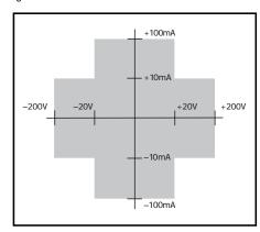
The Model 6430 provides four-quadrant sourcing of up to 2.2W, as well as measurement sensitivity down to sub-femtoamp and microvolt levels. It can measure currents from the 1pA range (with just 0.4fA p-p noise) up to the 100mA range at up to 20V. Voltage ranges from 200mV to 200V are available. Current and voltage range settings define the maximum source or sink voltage or current.
