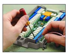
Screw terminals use oversize connectors for easier, mistake-free wiring. Easy-to-use removable terminals are available on some models.
