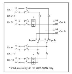
Scanner Configuration for Models 2000-SCAN and 2001-SCAN
