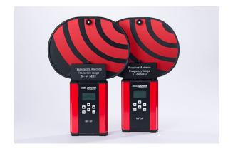
ETS-Lindgren's MF-9F Series of RF Leak Detector/Attenuation Meter Kits are designed to simplify the performance evaluation of shielding enclosures. These kits offer the ability to make measurements for military and commercial standards. The receiver module can store up to 63 attenuation levels per frequency to be downloaded to a PC. Windows compatible software is included for viewing, processing, and printing data.
