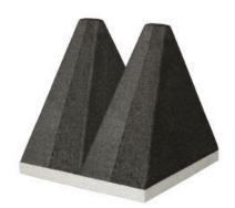
ETS-Lindgren's DuraSorb DSH-600H Absorber is the latest evolution of ETS-Lindgren's low profile, hybrid anechoic absorber technology. It combines the advantages of the proven FerroSorb performance with the physical properties of the PS Series absorbers. DuraSorb is constructed using substrates with rigid, closed cell foams, which are loaded volumetrically and uniformly throughout the absorbers. DSH-600H is ideal for 3 m range and 5 m range chambers.
