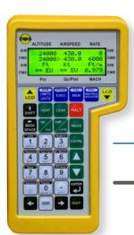
Optional Touch Screen Remote Control. Includes USB port for test program storage on USB memory
