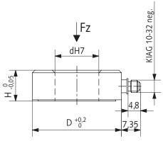
Fig. 1: Dimensions load washers
