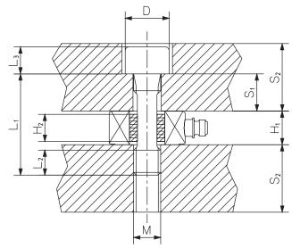
Fig. 2: Mounting with Type 9422A... (Included Accessories)
