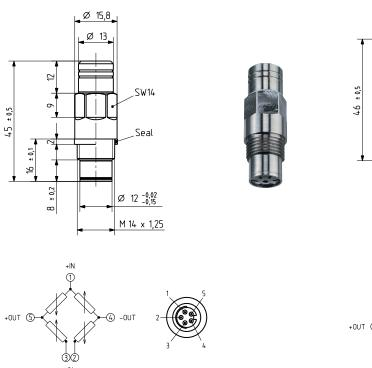
Fig. 1a: Sensor Bridge and Pin Allocation
