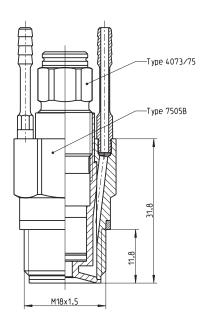
Fig. 4b: Mounting sensor Type 4075A... in cooling adapter Type 7505B
