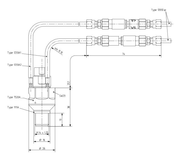
Fig. 5a: Switching adapter (water-cooled)Type 7533A...
