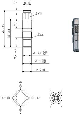
Fig. 1b: Sensor Bridge and Pin Allocation
