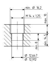
Fig. 3a: Mounting hole for Types 4043A.../4045A...
