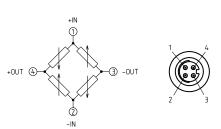
Fig. 2a: Sensor Bridge and Pin Allocation
