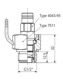
Fig. 4a: Mounting sensor Type 4045A... in damped cooling adapter Type 7511
