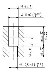
Fig. 3b: Mounting hole for Types 4073A.../4075A...
