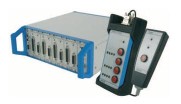
of an overload, the "Overload" condition of the measuring wheel connected is also indicated by LED on the Type 5617 RoaDyn module concerned.
