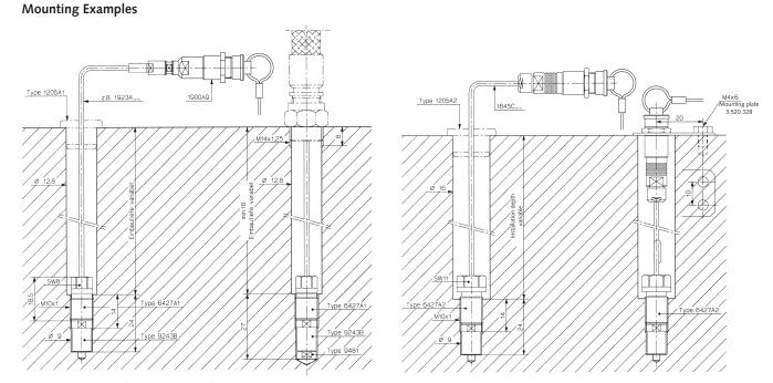
Fig. 6: Examples of different methods of mounting Type 9243B longitudinal measuring pin
