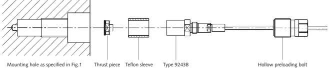
Hollow preloading bolt (requires 8 mm wrench)
