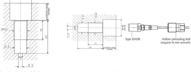
Fig. 1: Mounting hole with flat bottom
