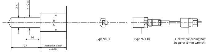
Fig. 3: Mounting hole with conical bottom
