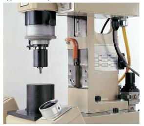
Fig. 1: Measuring force-proportional strain on a wobble riveting machine (C-form construction)
