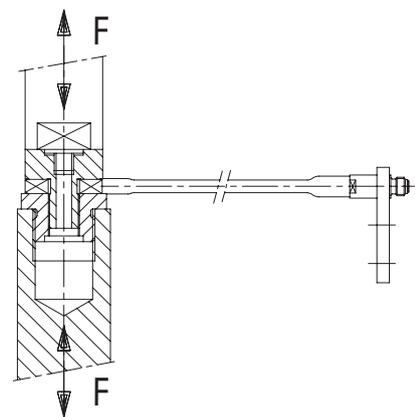
Measurement of tension and compression forces. Used in combination with hydraulic cylinders, for example.
