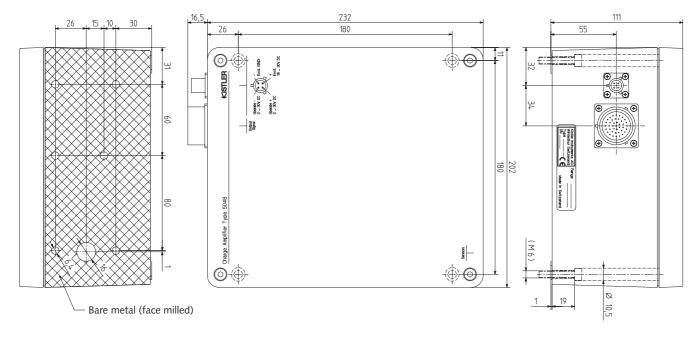
Fig. 2: Multi-channel charge amplifiers Type 5048A... (16, 24 or 32 channels)
