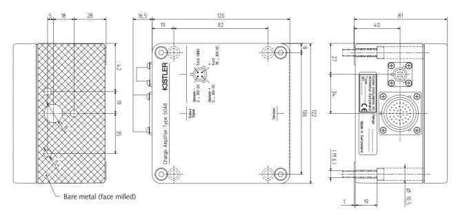
Fig. 1: 8-channel charge amplifiers Type 5048A...
