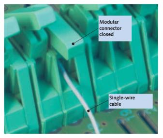
Connecting single-wire cable to charge amplifier module
