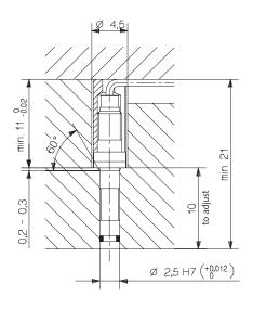
Fig. 3: Installation with spacer sleeve Type 6464
