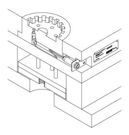
Fig. 4: Sensor, cable, mounting plate and identification plate
