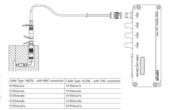
Fig. 2: Sensor Type 6155AE with charge amplifier Type 5155A... (1-, 2- or 4-channel; SmartAmp optional on one channel)
