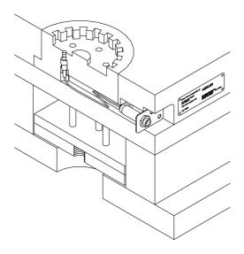
Fig. 7: Sensor, cable, connector, mounting plate and identification plate
