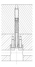
Fig. 4: Installation with 50 mm extension and holding plate
