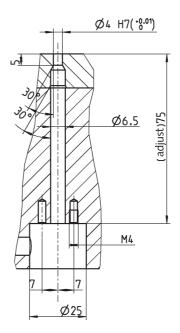
Fig. 6: Bore dimension for Type 6155AE with extension sleeve and holding plate
