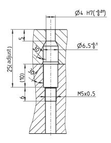
Fig. 5: Bore dimension Type 6155AE
