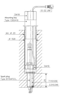
Fig. 1: Mounting of the measuring spark plug
