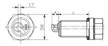
Fig. 2: Spark plug dimensions
