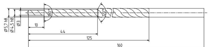
Fig. 11: Step drill Type 1300A16
