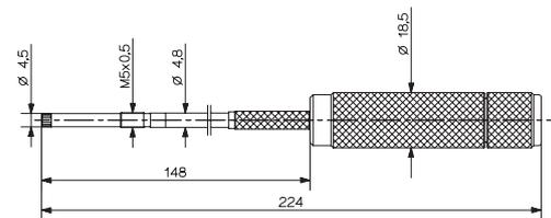
Fig. 10: Reaming tool Type 1300A99
