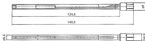
Fig. 7: Mounting key ø5,6 mm, slotted, Type 1300B14
