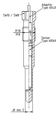
Fig. 3: Mounting in glow plug adapter
