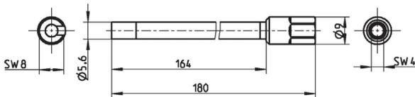
Fig. 5: Mounting key Type 1300A14
