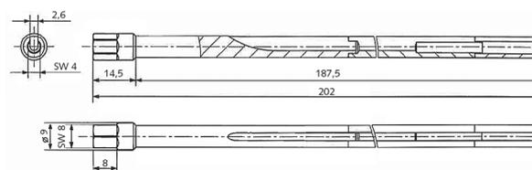
Fig. 8: Mounting key ø7,3 mm, slotted, Type 1300B14Q01
