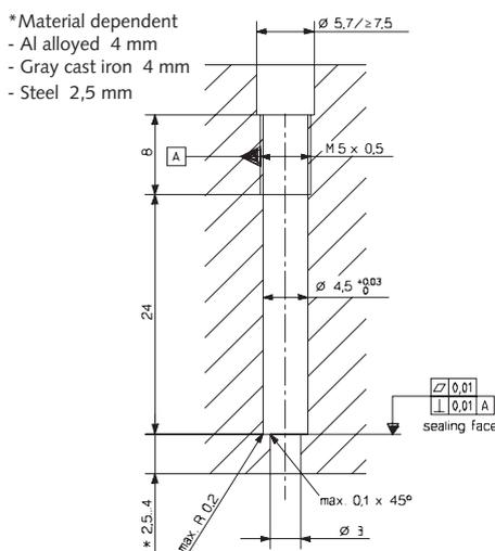
Fig. 1: Dimensions of the mounting bore
