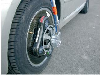
Fig. 1: Out-board transmission module on the RoaDyn® S625 System 2000 measuring wheel
