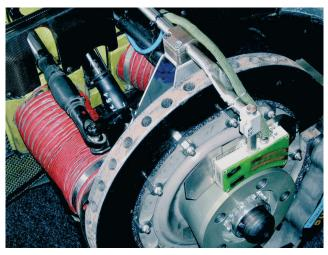
Fig. 2: Stator mounted on vehicle
