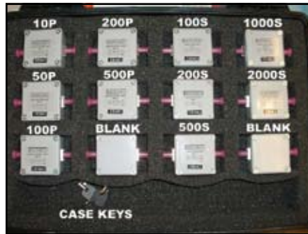
10 resistors (+ 2 blanks) in the kit
